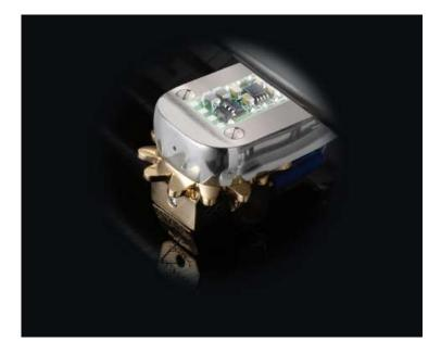
The **Clearaudio** Absolute Phono is the world's first active headshell moving coil phonostage. A tiny circuit board installed in the headshell of the tonearm amplifies the highly sensitive moving coil cartridge signal at its source. As a result, the signal to noise ratio is improved by approximately ten decibels across the entire audio bandwidth.
