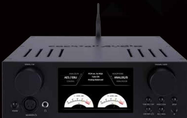
The HA500H is a premium Hybrid Headphone Amplifier, DAC, Pre-Amplifier and Asynchronous USB DAC for audiophiles. It is equipped with two(2) ECC82 vacuum tubes and solid state OP Amp, which will work as preamp stage for the headphone section, and will work as out stage for the pre-out section, while solid state transistors are built in at power amp stage for headphone section. So, you can select one out of Tube and OP Amp according to character of music, your feelings and mood.
