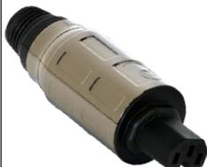
**Description:** Standard 15 amp IEC designed for large diameter power cables with heavy gauge conductors. The non-magnetic anti-resonant shell is plated and clear coated to help reject RFI/EMI noise. Recommended cable diameter: 7.5mm/.29" to a maximum of 21.5mm/.84"
