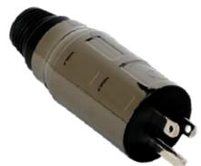
**Description:** Standard North American power plug designed for large diameter power cables with heavy gauge conductors. The non-magnetic anti-resonant shell is plated and clear coated to help reject RFI/EMI noise. Recommended cable diameter: 7.5mm/.29" to a maximum of 21.5mm/.84"
