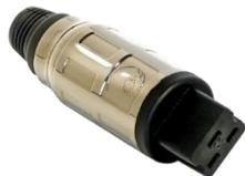
**Description:** 20 amp IEC designed for large diameter power cables with heavy gauge conductors. The non-magnetic anti-resonant shell is plated and clear coated to help reject RFI/EMI noise. Not intended for use on wimpy power cables. Recommended cable diameter: 7.5mm/.29" to a maximum of 21.5mm/.84"
