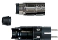
**Description:** European Schuko power plug designed for large diameter power cables with heavy gauge conductors. The non-magnetic anti-resonant shell is plated and clear coated to help reject RFI/EMI noise. Recommended cable diameter: 7.5mm/.29" to a maximum of 21.5mm/.84"
