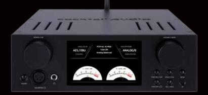
The HA500H is a premium Hybrid Headphone Amplifier, DAC, Pre-Amplifier and Asynchronous USB DAC for audiophiles. It is equipped with two(2) ECC82 vacuum tubes and solid state OP Amp, which will work as preamp stage for the headphone section, and will work as out stage for the pre-out section, while solid state transistors are built in at power amp stage for headphone section. So, you can select one out of Tube and OP Amp according to character of music, your feelings and mood.
