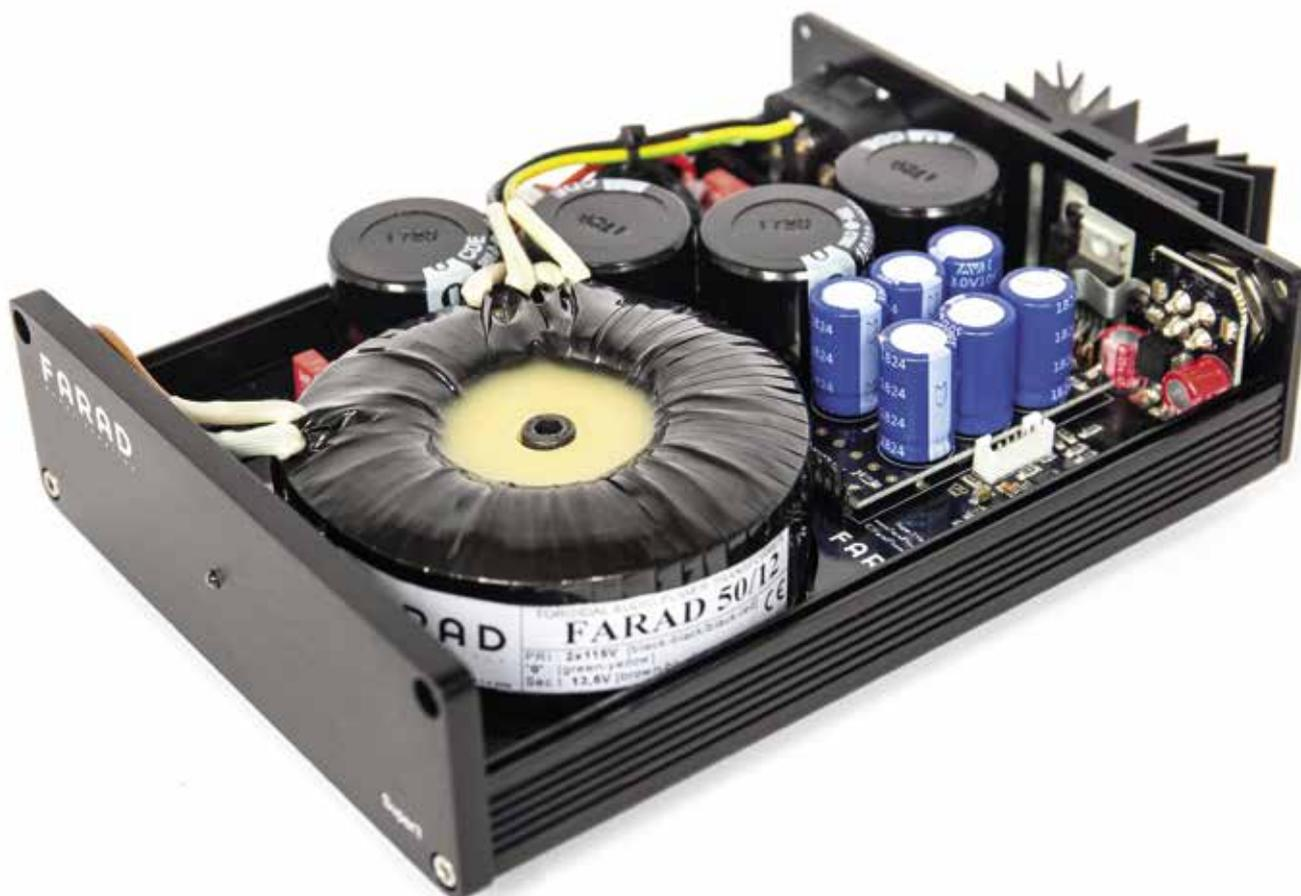
▶ (there's a reset button on the rear panel). The Super3 is, in effect, a dual-regulation power supply, the first – which already makes a good power supply in its own right – charges the supercapacitor bank, while the second provides regulated output voltage and current from this supercapacitor bank, which acts as a sort of active battery.
