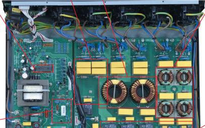
Filter for switch mode power supplies with high level filtering
